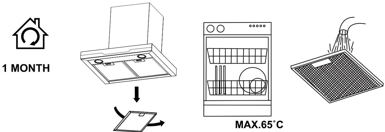
**Aluminium filters:** To avoid fires, clean thoroughly once a month or whenever the display pilot light lights up (if fitted). To do so, remove the filters and soak in hot water and detergent for an hour. If using a dishwasher, position the filters vertically to improve the cleaning process.
